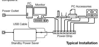
The Accessory devices should all be plugged into a Power-Strip and plugged into the Female Power Socket of the Product. The Male Power Plug should plug directly into a wall Power Outlet. Care should be taken to ensure that the computer / CPU / PC is plugged into a separate power outlet directly. The product will not work correctly if the PC is plugged into the power-strip controlled
